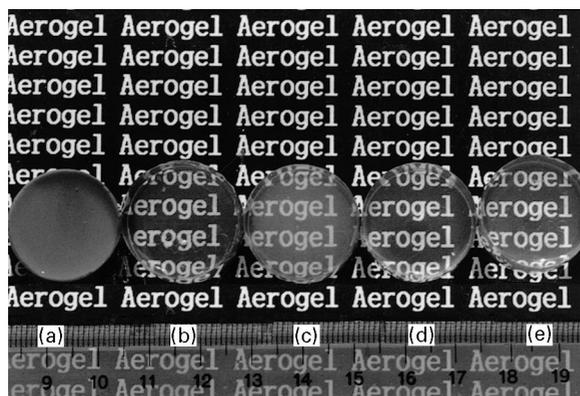
Figure 11 Photograph of the monolithic aerogels in the TMOS-based systems (All specimens are 1 cm in thickness.); (A) M6AB, (B) M3AA1, (C) M6AA, (D) M3AA2 and (E) M3AA3.
